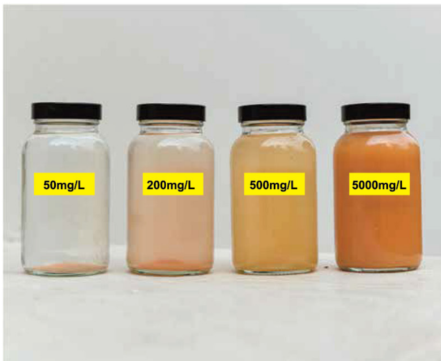
Measurement of Total Suspended Solids (TSS) in mg/l
