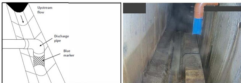
Figure 2. Example of Blue-Marker painted on cut-opened discharge pipe.
